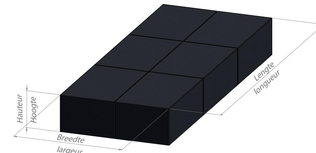
**2X (LENGTE + BREEDTE) X HOOGTE = INFILTRATIEOPPERVLAKTE (M<sup>2</sup>)**
