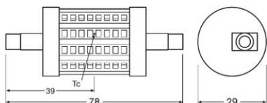
LINE 78.0 mm 60 7 W/2700K R7s, LINE 78.0 mm 75 8 W/2700K R7s
