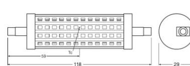
LINE 118.0 mm 100 12.5 W/2700K R7s, ST LINE 118.0 mm 125 15 W/2700K R7s
